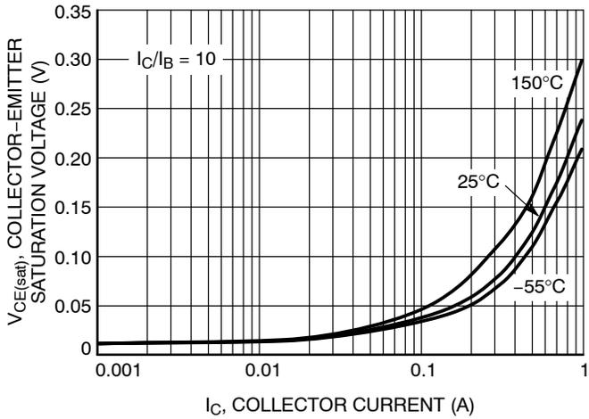
**Figure 3. Collector Emitter Saturation Voltage vs. Collector Current**
