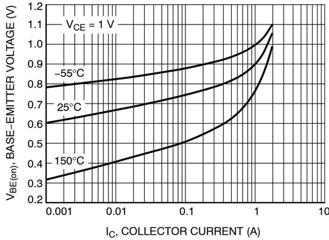
**Figure 5. Base Emitter Voltage vs. Collector Current**
