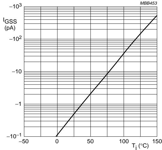
$V_{DS} = 0$ ;  $V_{GS} = -20$  V.
