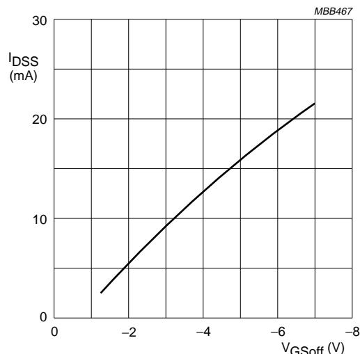
$V_{DS} = 15 \text{ V}; T_j = 25^\circ\text{C}$ .
