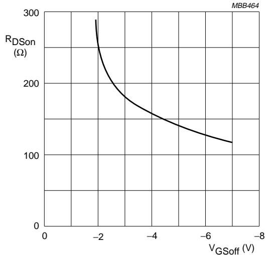
$V_{DS} = 100 \text{ mV}; V_{GS} = 0; T_j = 25^\circ\text{C}$ .
