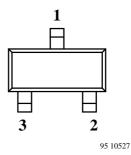
BF550 Marking: LA Plastic case (SOT 23) 1= Collector; 2= Base; 3= Emitter
