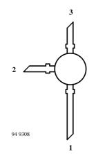
BF979 Marking: BF979 Plastic case (TO 50) 1= Collector; 2= Base; 3= Emitter
