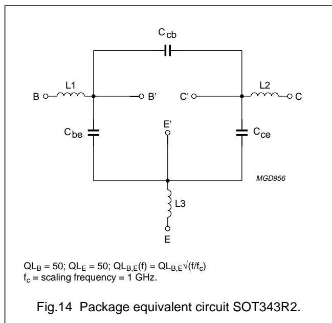
Fig.14 Package equivalent circuit SOT343R2.
