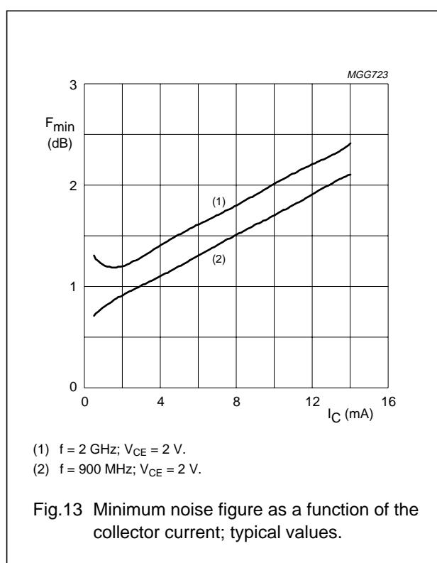
Fig.13 Minimum noise figure as a function of the collector current; typical values.
