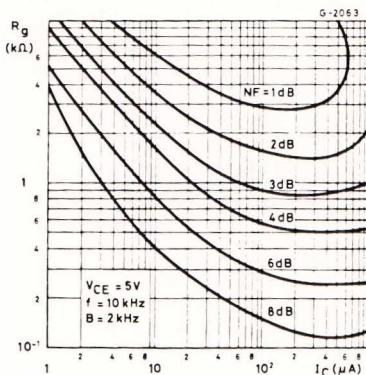
Contours of Constant Noise Figure  $f = 1\text{kHz}$ .
