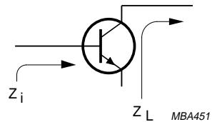
Fig.16 Definition of transistor impedance.
