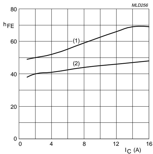
Measured under pulsed conditions;  $t_p \leq 300 \mu\text{s}$ ;  $\delta \leq 0.01$ .(1)  $V_{\text{CE}} = 26 \text{ V}$ .(2)  $V_{\text{CE}} = 10 \text{ V}$ .
