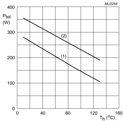
Total device; both sections equally loaded.
