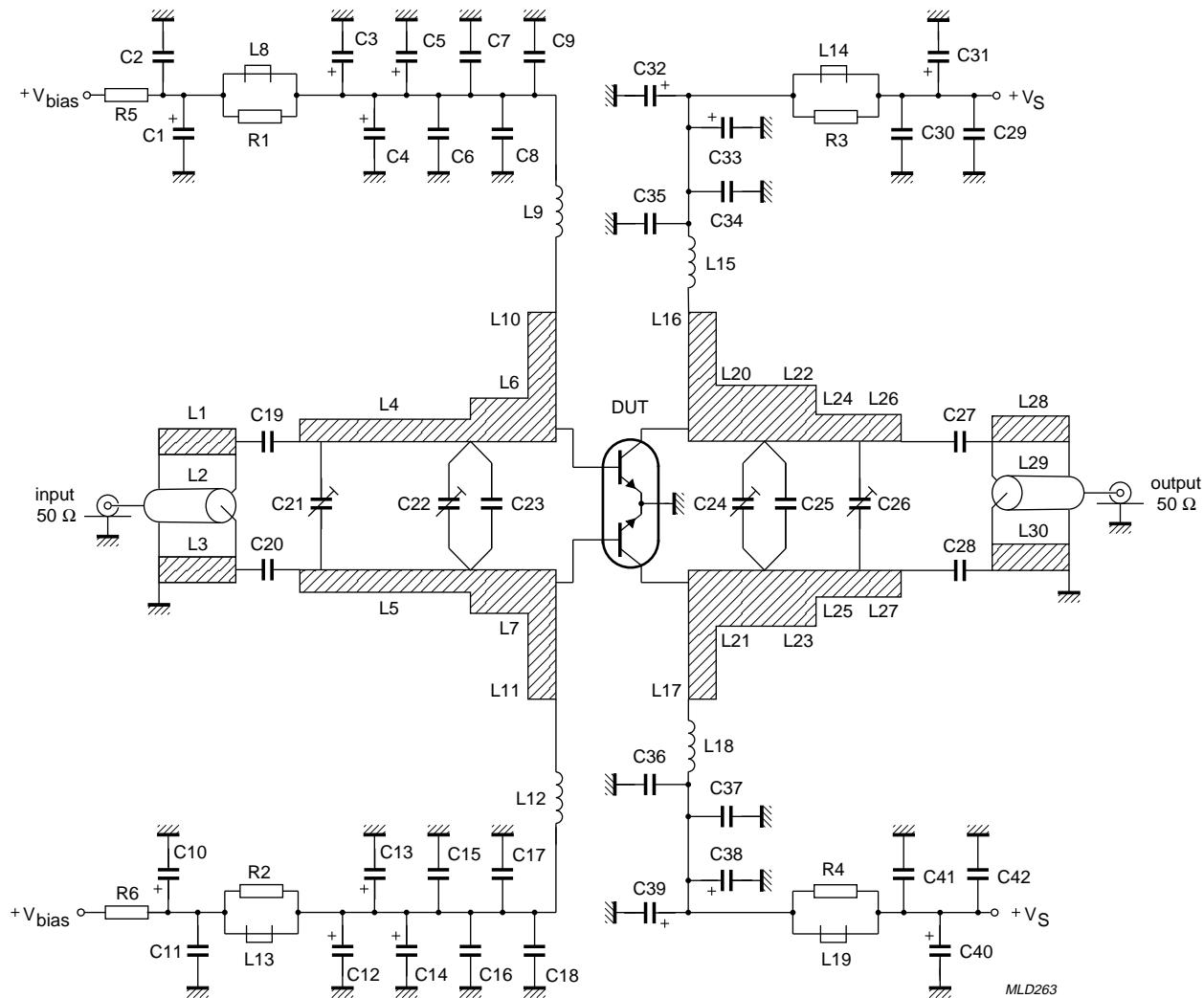
Fig.11 Class-AB test circuit at 900 to 960 MHz.
