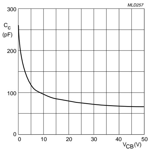
Value  $C_c$  is that of the die only, it is not measurable because of internal matching network. $I_E = i_e = 0$ ;  $f = 1 \text{ MHz}$ .
