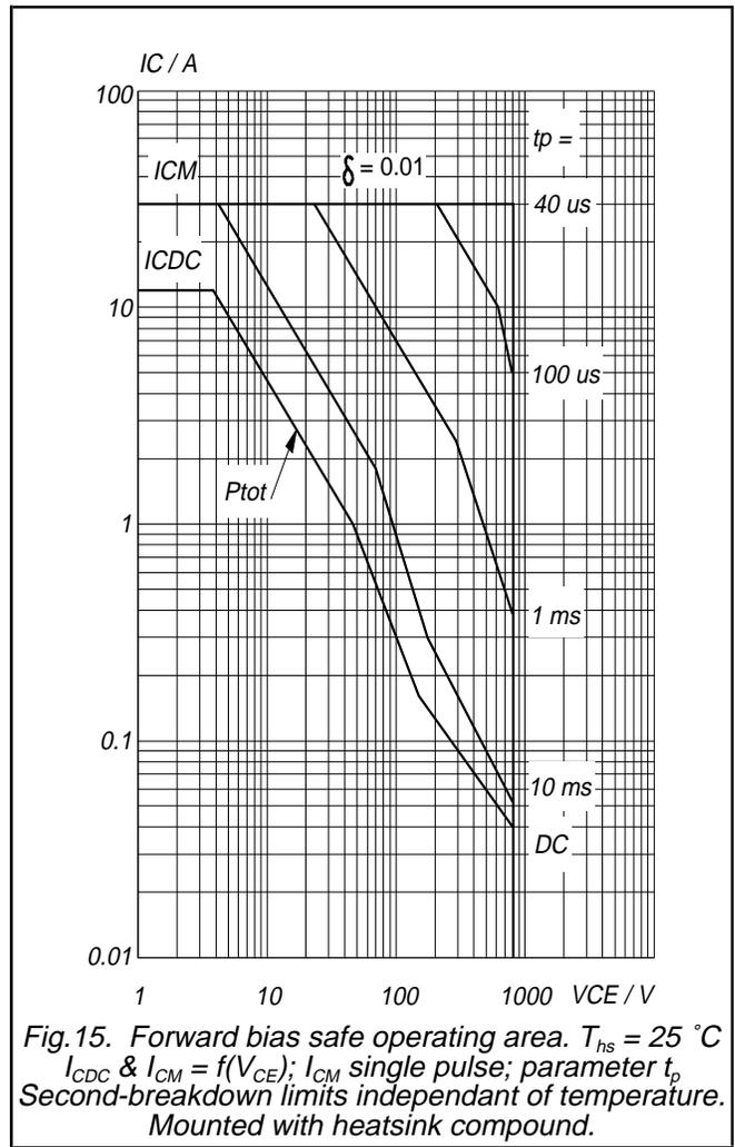
Silicon Diffused Power Transistor
