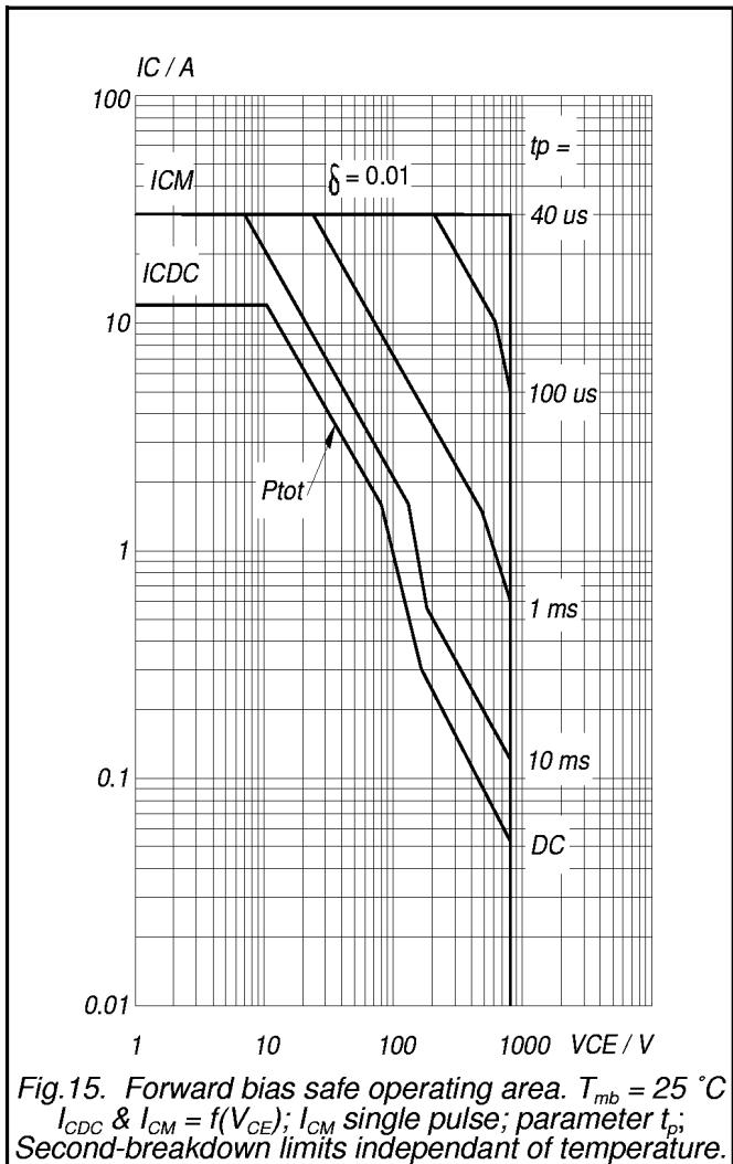
Fig.15. Forward bias safe operating area.  $T_{mb} = 25^\circ\text{C}$
