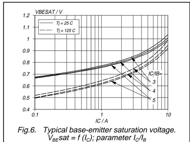
Silicon Diffused Power Transistor
