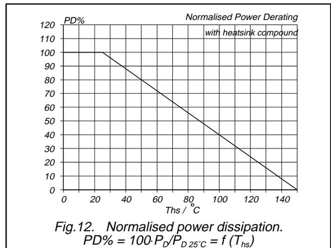
Silicon Diffused Power Transistor
