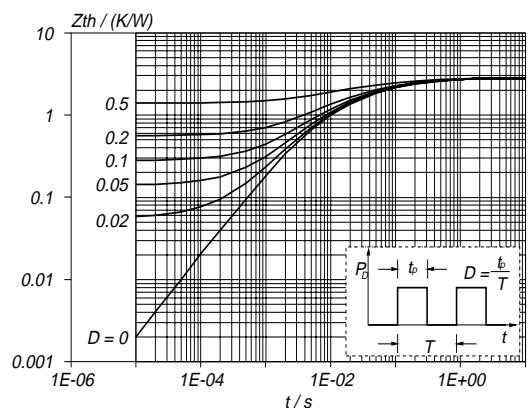
Fig.14. Transient thermal impedance.
