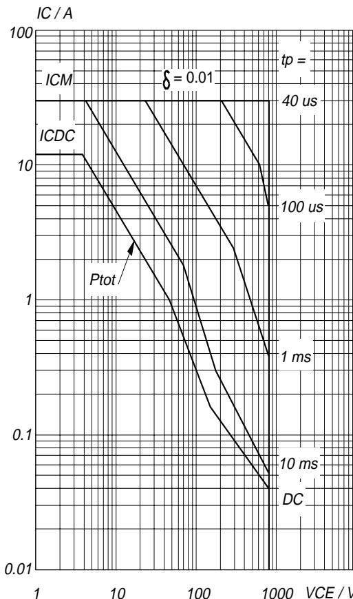
Fig.15. Forward bias safe operating area.  $T_{hs} = 25^\circ C$
