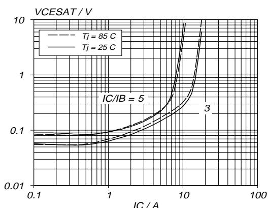
Fig.9. Typical collector-emitter saturation voltage.
