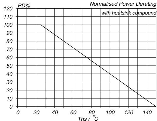
Fig.13. Normalised power dissipation.
