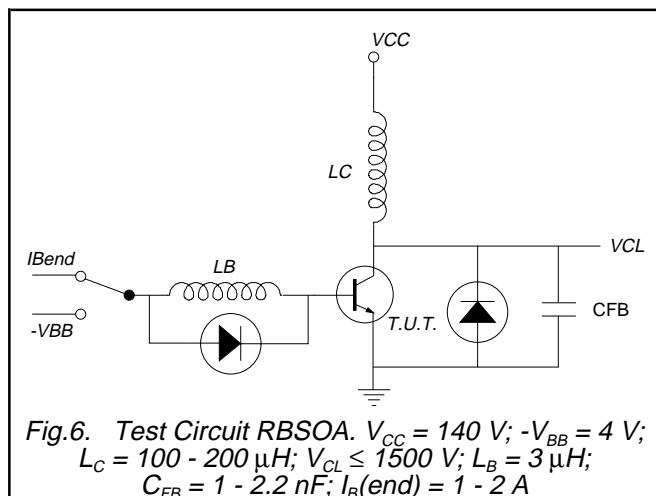
Fig.6. Test Circuit RBSOA.  $V_{CC} = 140 \text{ V}$ ;  $-V_{BB} = 4 \text{ V}$ ;  $L_C = 100 - 200 \mu\text{H}$ ;  $V_{CL} \leq 1500 \text{ V}$ ;  $L_B = 3 \mu\text{H}$ ;  $C_{FB} = 1 - 2.2 \text{ nF}$ ;  $I_B(\text{end}) = 1 - 2 \text{ A}$
