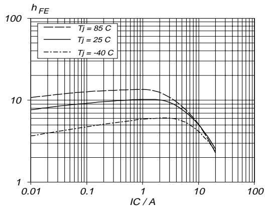
Fig.7. Typical DC current gain.  $h_{FE} = f(I_C)$
