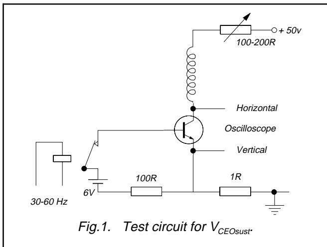
Fig.1. Test circuit for  $V_{CEO}sust$ .
