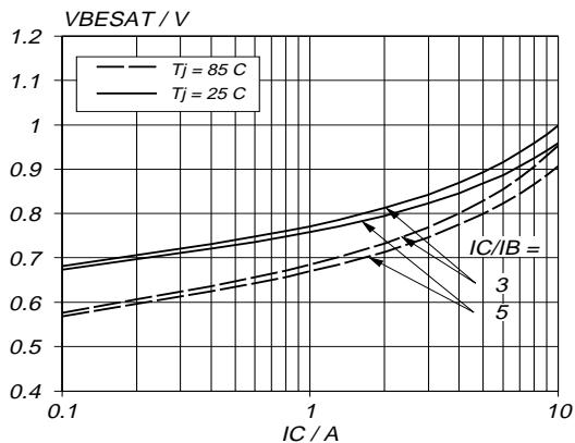
Fig.8. Typical base-emitter saturation voltage.
