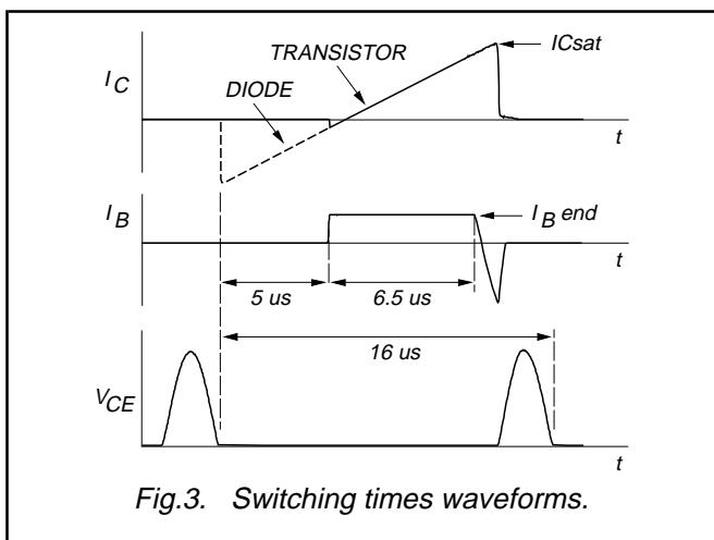
Fig.3. Switching times waveforms.
