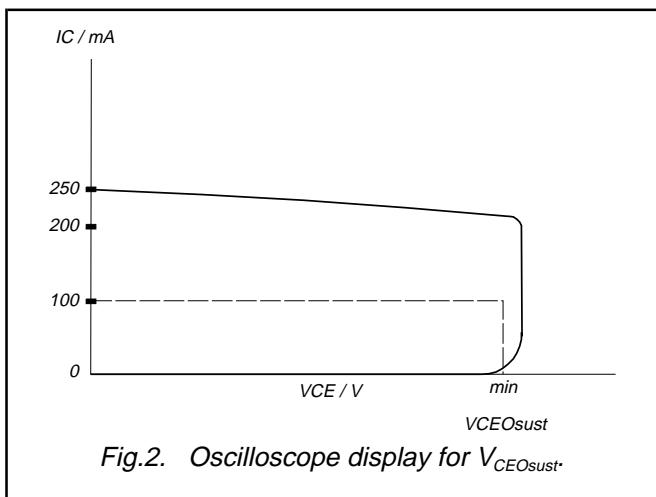
Fig.2. Oscilloscope display for  $V_{CEO}sust$ .
