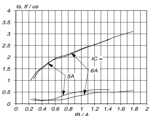
Fig.12. Typical collector storage and fall time.
