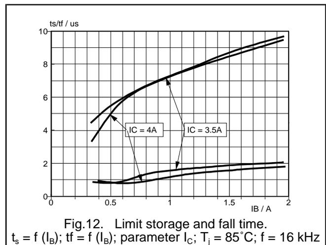
Silicon Diffused Power Transistor
