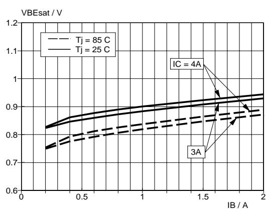
Fig.7. Typical base-emitter saturation voltage.
