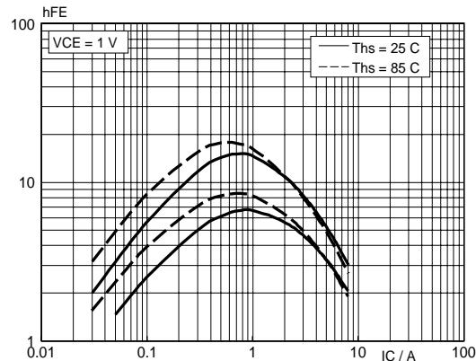
Fig.5. DC current gain,  $h_{FE} = f(I_C)$
