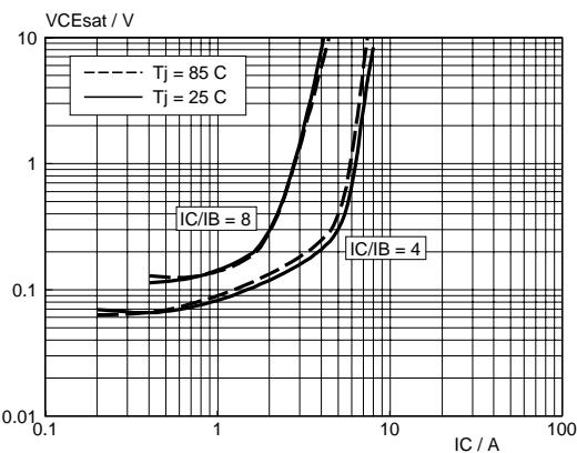
Fig.6. Typical collector-emitter saturation voltage.
