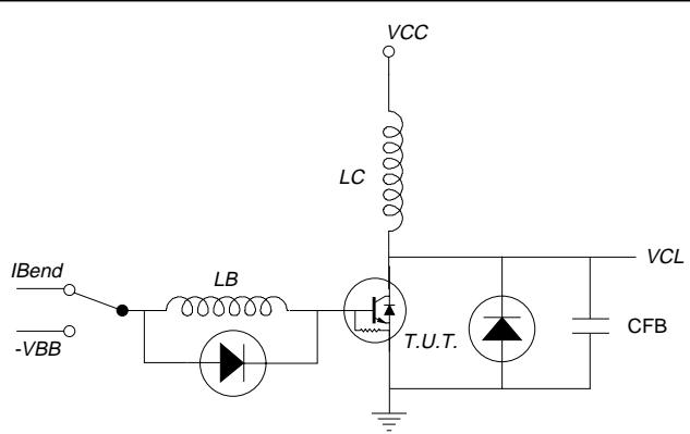
Fig.13. Test Circuit RBSOA.  $V_{CC} = 150$  V;
