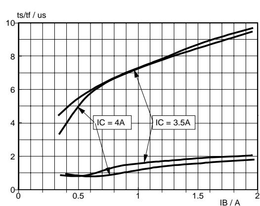
Fig.10. Limit storage and fall time.
