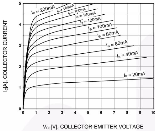
Figure 1. Static Characteristic
