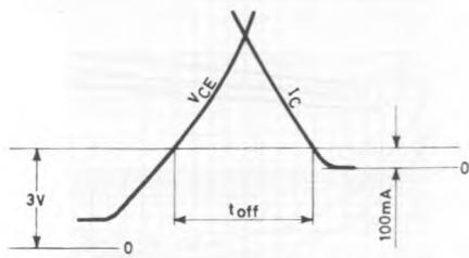
Turn-off time is the time for the collector current  $I_C$  to decrease to 100mA after the collector to emitter voltage  $V_{CE}$  has risen 3V into its flyback excursion
