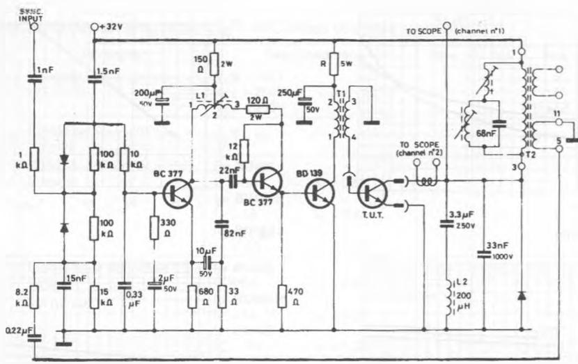
L1 Horizontal hold coil : Pins 1-2 = 75 turns Ø 0.2mm ; R = 1.5Ω ; L min = 0.62mH
