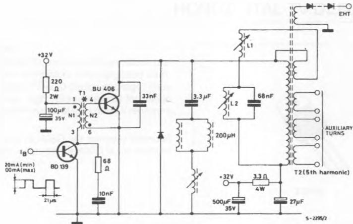
\* N1 = 125 turns Ø 0.3mm ; N2 = 30 turns Ø 0.6mm ; GAP = 0.12mm ; CORE = DOUBLE E 19x5x8mm ; FERRITE 3E1 TYPE
