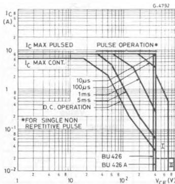
I = Area of permissible operation driving turn-on provided  $R_{BE} = 100\Omega$  and  $t_p \leq 0.6 \mu s$ .
