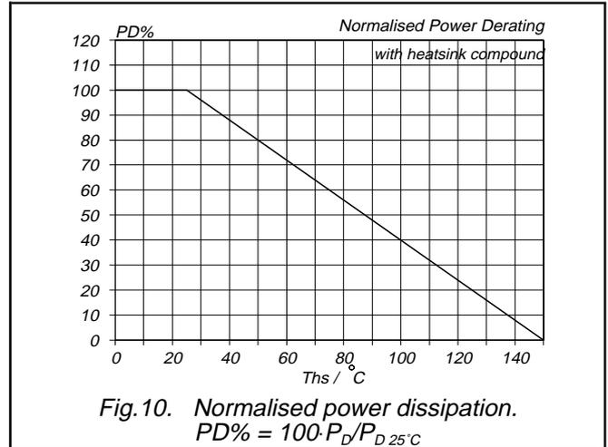
Fig.10. Normalised power dissipation.
