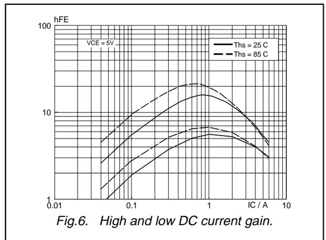
Fig.6. High and low DC current gain.
