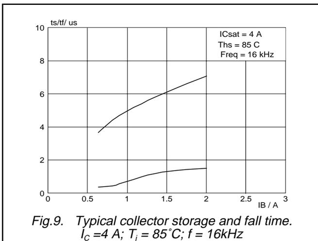
Fig.9. Typical collector storage and fall time.
