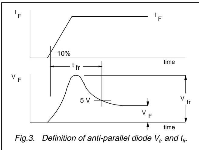
Fig.3. Definition of anti-parallel diode Vfr and tfr.
