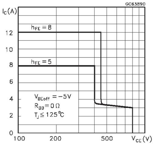
RBSOA and Inductive Load Switching Test Circuit
