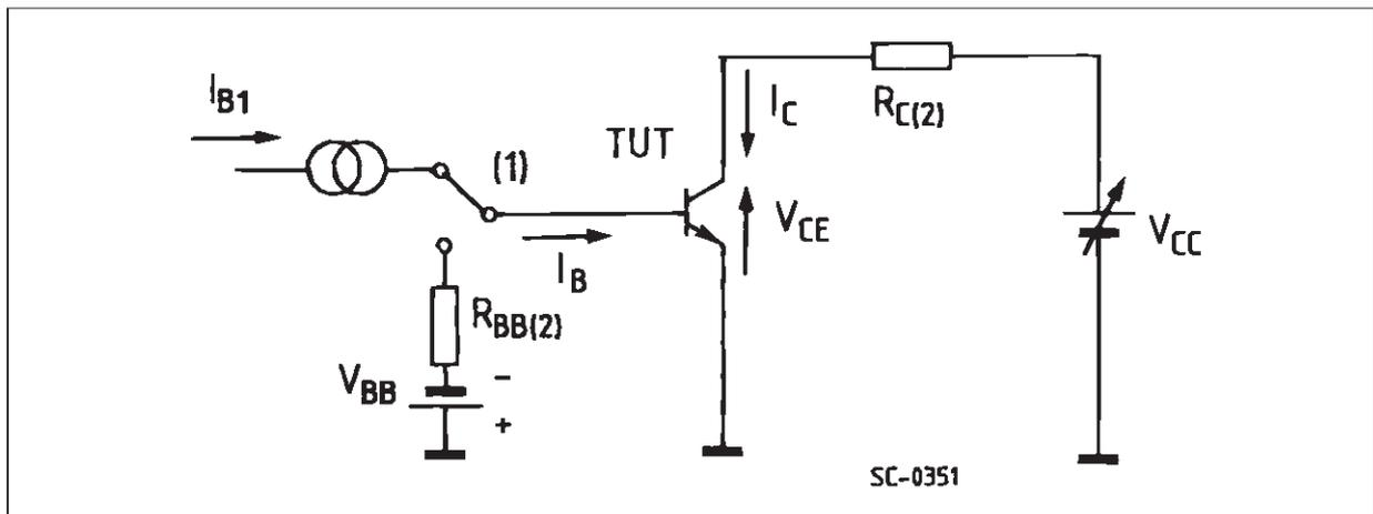
Energy Rating Test Circuit
