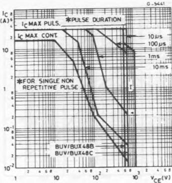
I - Area of permissible operation during turn-on provided  $R_{BE} \leq 100 \Omega$  and  $t_p \leq 0.2 \mu s$ .
