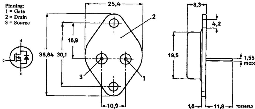
Fig.1 TO3; drain connected to mounting base.
