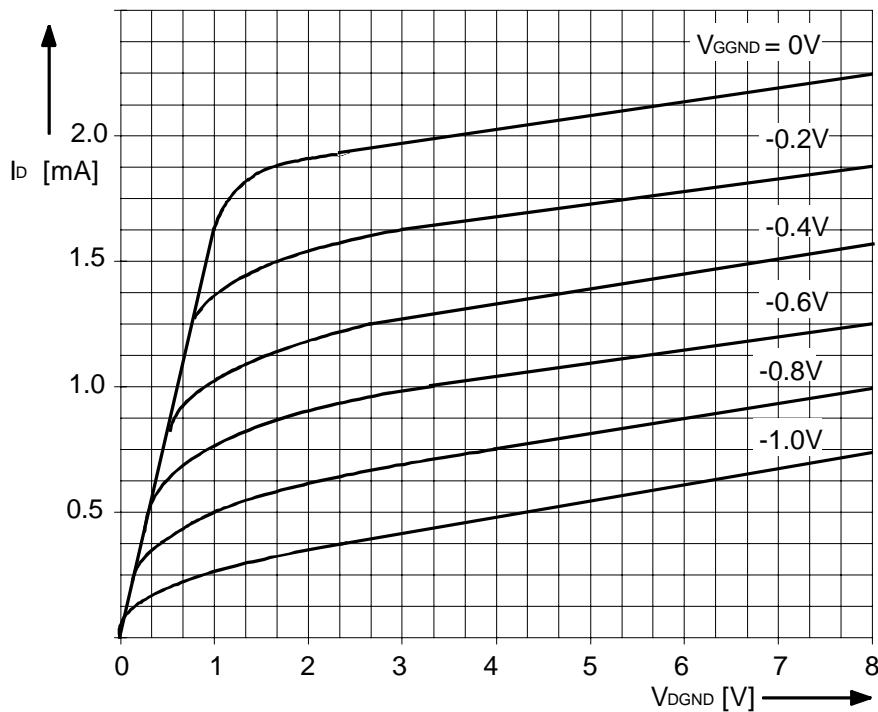
**Output characteristics  $I_D = f(V_{DS})$ , S connected to GND.**
