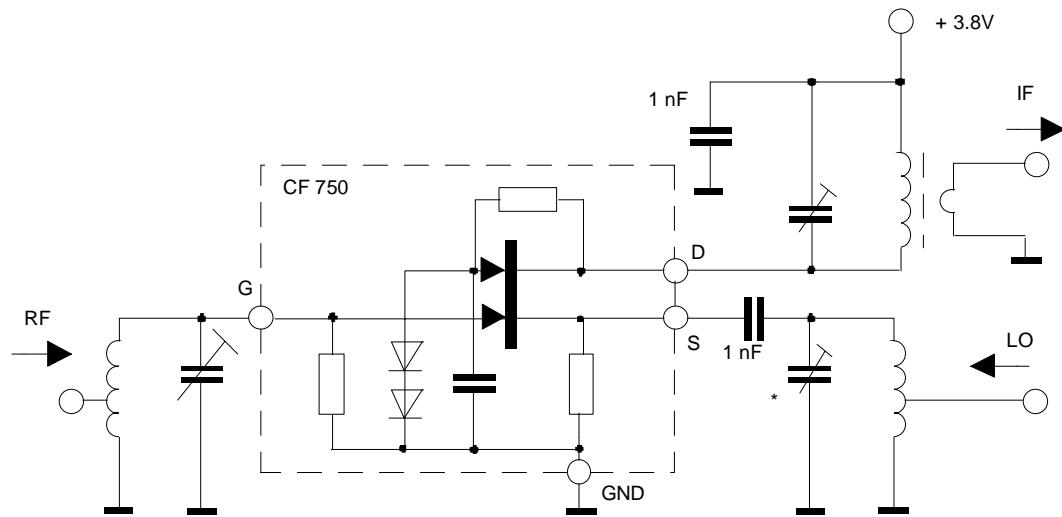
\* must be high capacitance to ensure good IF grounding at source
