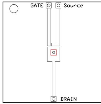
Max  $R_{\theta JA} = 162^{\circ}\text{C/W}$
