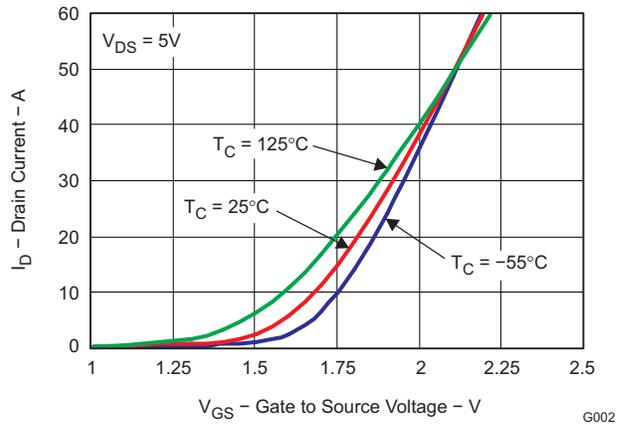
**Figure 3. Transfer Characteristics**
