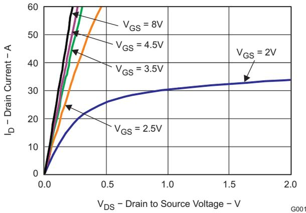
**Figure 2. Saturation Characteristics**
