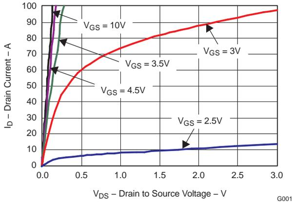
**Figure 2. Saturation Characteristics**
