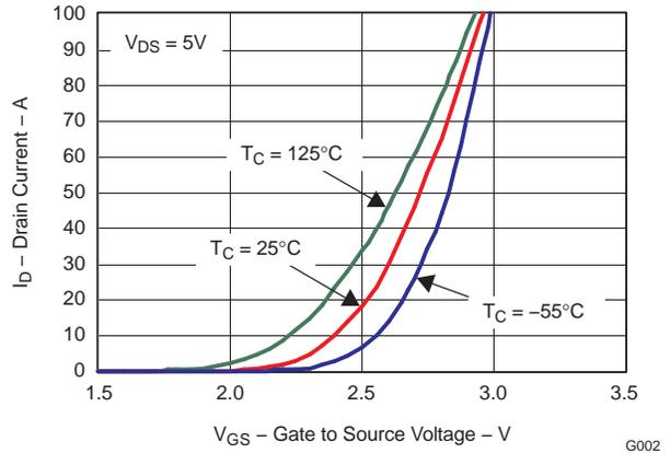
**Figure 3. Transfer Characteristics**
