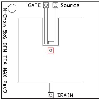
Max  $R_{\theta JA} = 53^{\circ}\text{C/W}$
