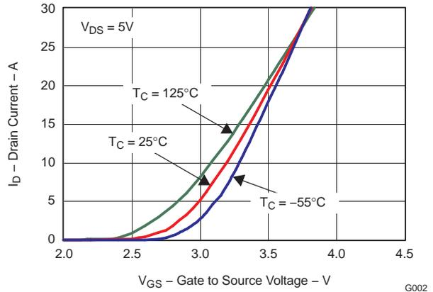
**Figure 3. Transfer Characteristics**
