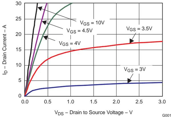
**Figure 2. Saturation Characteristics**
