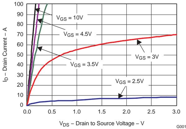
**Figure 2. Saturation Characteristics**
