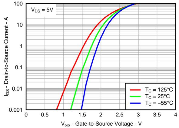
**Figure 3. Transfer Characteristics**
