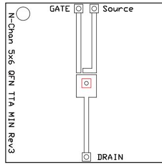
Max  $R_{\theta JA} = 120^{\circ}\text{C/W}$
