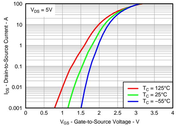
**Figure 3. Transfer Characteristics**
