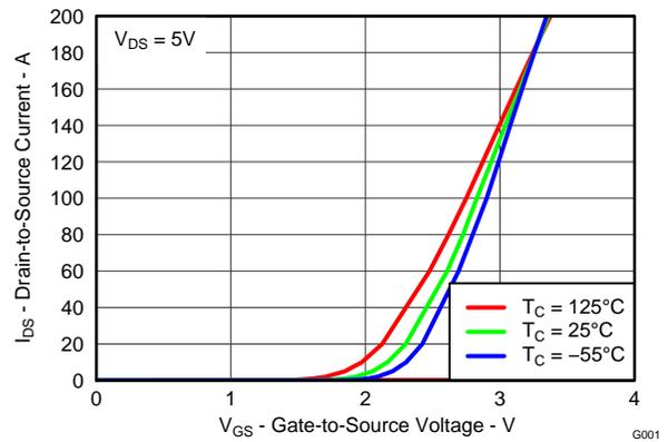
**Figure 3. Transfer Characteristics**
