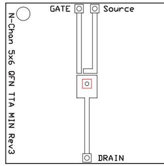
Max  $R_{\theta JA} = 122.4^{\circ}\text{C/W}$
