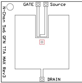
Max  $R_{\theta JA} = 50.6^{\circ}\text{C/W}$
