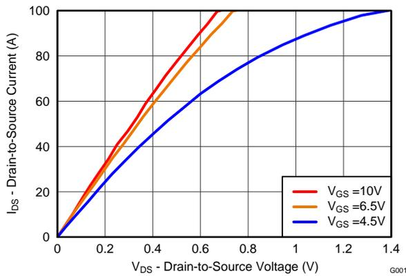
Figure 2. Saturation Characteristics
