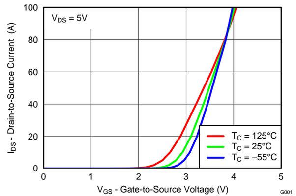
Figure 3. Transfer Characteristics
