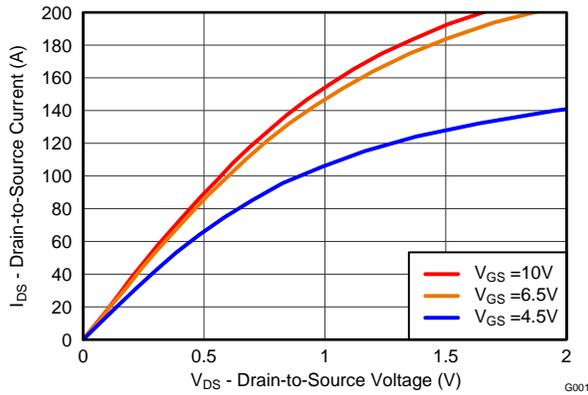
**Figure 3. Saturation Characteristics**
