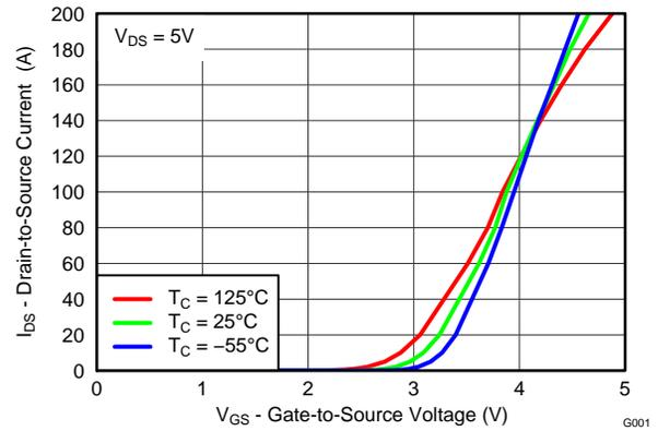
**Figure 4. Transfer Characteristics**
