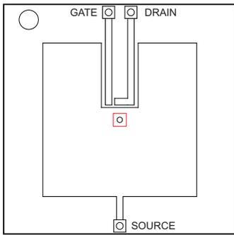
Max  $R_{\theta JA} = 63^{\circ}\text{C/W}$
