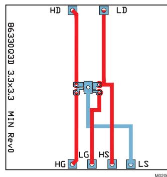
Max  $R_{\theta JA} = 135^\circ\text{C/W}$  when mounted on minimum pad area of 2-oz. (0.071-mm thick) Cu.
