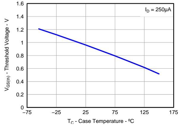
**Figure 19. Sync MOSFET V<sub>GS(th)</sub>**
