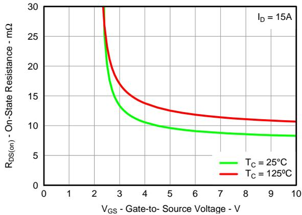
**Figure 20. Control MOSFET R<sub>DS(on)</sub> vs V<sub>GS</sub>**
