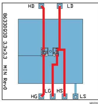
Max  $R_{\theta JA} = 73^\circ\text{C/W}$  when mounted on 1 inch<sup>2</sup> (6.45 cm<sup>2</sup>) of 2-oz. (0.071-mm thick) Cu.
