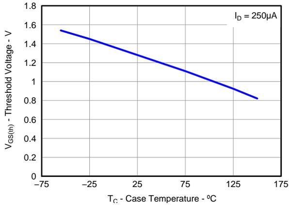
**Figure 18. Control MOSFET V<sub>GS(th)</sub>**
