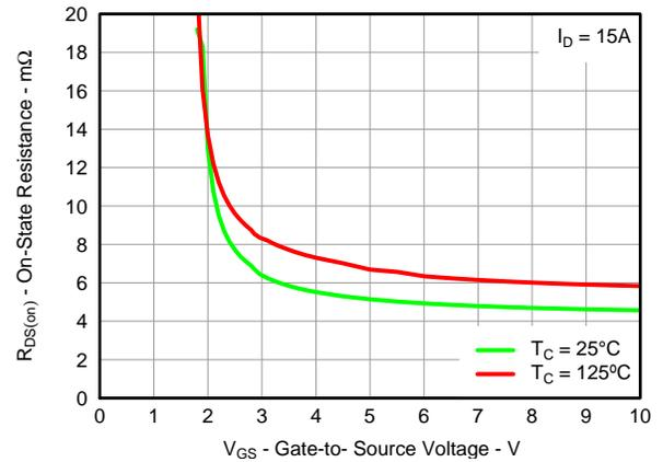
**Figure 21. Sync MOSFET R<sub>DS(on)</sub> vs V<sub>GS</sub>**
