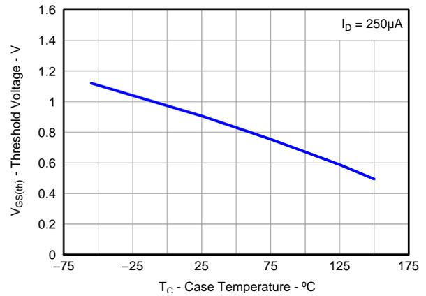
**Figure 19. Sync MOSFET V<sub>GS(th)</sub>**
