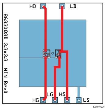
Max  $R_{\theta JA} = 80^\circ\text{C/W}$  when mounted on 1 inch<sup>2</sup> (6.45 cm<sup>2</sup>) of 2-oz. (0.071-mm thick) Cu.
