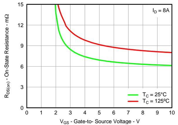
**Figure 21. Sync MOSFET R<sub>DS(on)</sub> vs V<sub>GS</sub>**
