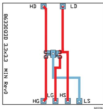
Max  $R_{\theta JA} = 149^\circ\text{C/W}$  when mounted on minimum pad area of 2-oz. (0.071-mm thick) Cu.
