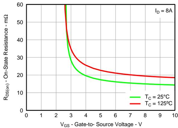
**Figure 20. Control MOSFET R<sub>DS(on)</sub> vs V<sub>GS</sub>**
