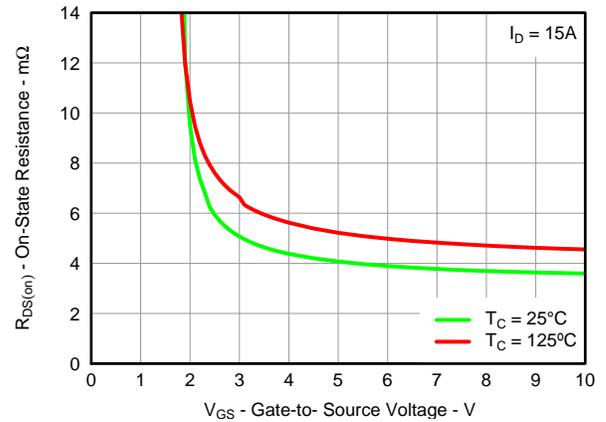
Figure 21. Sync MOSFET R<sub>DS(on)</sub> vs V<sub>GS</sub>
