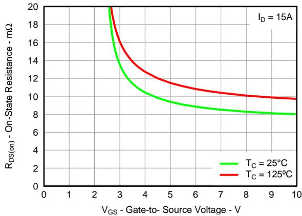
Figure 20. Control MOSFET R<sub>DS(on)</sub> vs V<sub>GS</sub>
