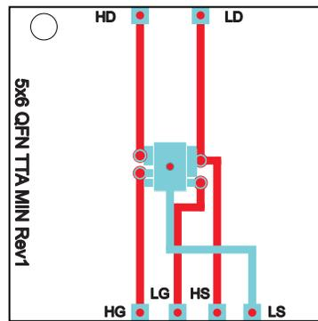
Max R<sub>θJA</sub> = 150°C/W when mounted on minimum pad area of 2-oz. (0.071-mm thick) Cu.
