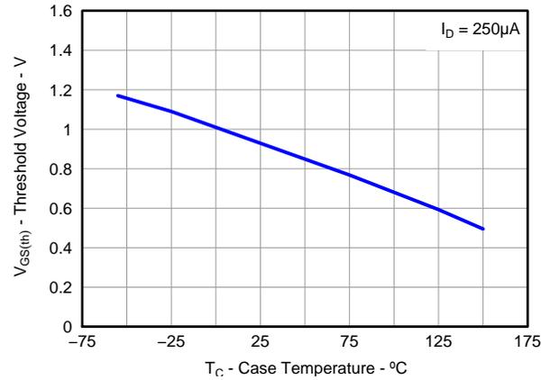
Figure 19. Sync MOSFET V<sub>GS(th)</sub>
