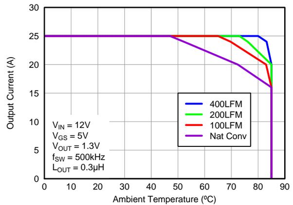
Figure 4. Safe Operating Area – PCB Horizontal Mount<sup>(1)</sup>
