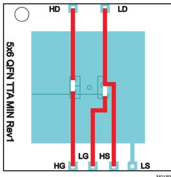
Max R<sub>θJA</sub> = 82°C/W when mounted on 1 inch<sup>2</sup> (6.45 cm<sup>2</sup>) of 2-oz. (0.071-mm thick) Cu.
