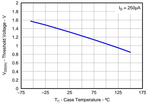
Figure 18. Control MOSFET V<sub>GS(th)</sub>
