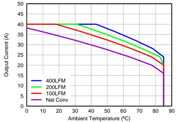
Figure 4. Safe Operating Area – PCB Horizontal Mount<sup>(1)</sup>
