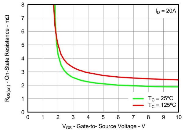
**Figure 21. Sync MOSFET R<sub>DS(on)</sub> vs V<sub>GS</sub>**
