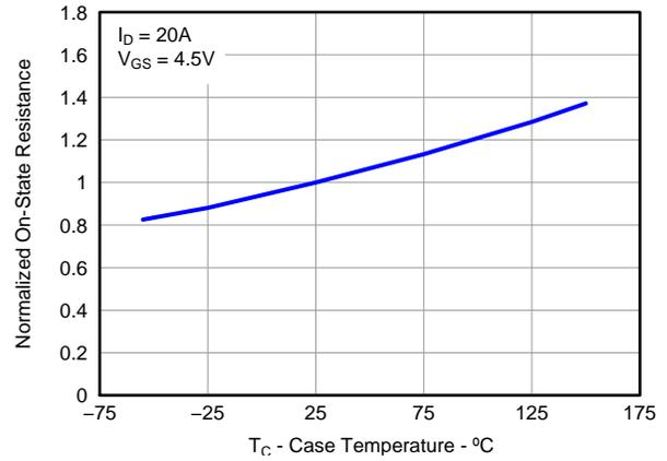
**Figure 23. Sync MOSFET Normalized R<sub>DS(on)</sub>**
