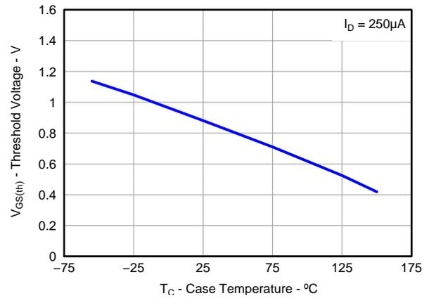
**Figure 19. Sync MOSFET V<sub>GS(th)</sub>**
