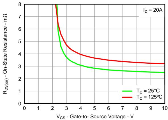
**Figure 20. Control MOSFET R<sub>DS(on)</sub> vs V<sub>GS</sub>**
