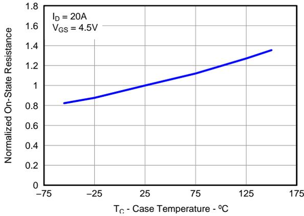
**Figure 22. Control MOSFET Normalized R<sub>DS(on)</sub>**
