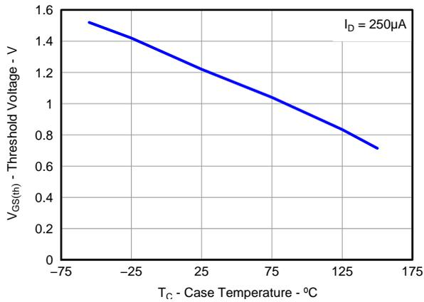
**Figure 18. Control MOSFET V<sub>GS(th)</sub>**
