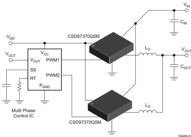
Figure 1. Application Diagram
