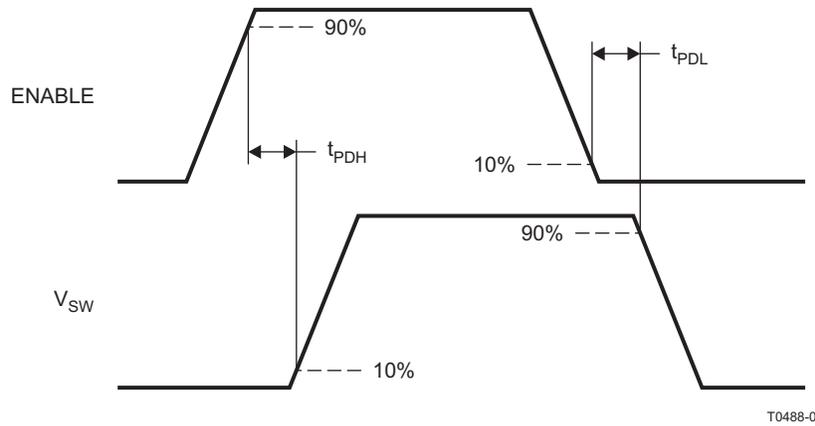
Figure 5. CSD97370Q5M ENABLE Timing Diagram ( $V_{DD} = PWM = 5V$ )
