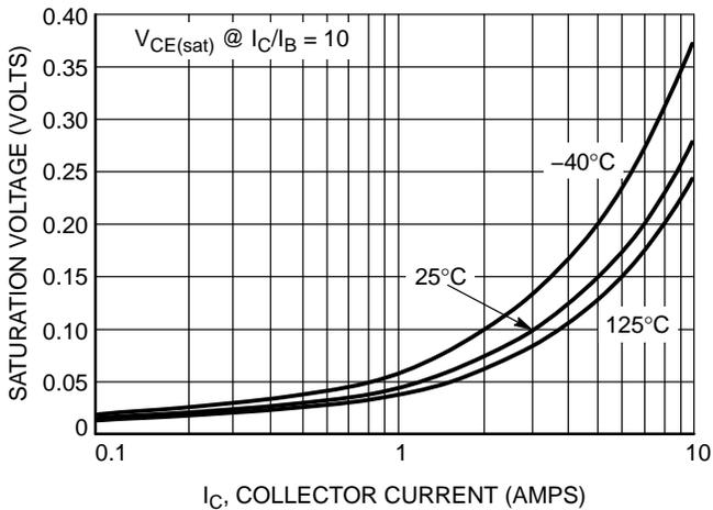
**Figure 5. D44H11 ON-Voltage**
