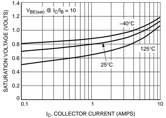
**Figure 8. D45H11 ON-Voltage**
