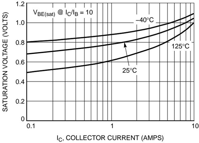
**Figure 7. D44H11 ON-Voltage**
