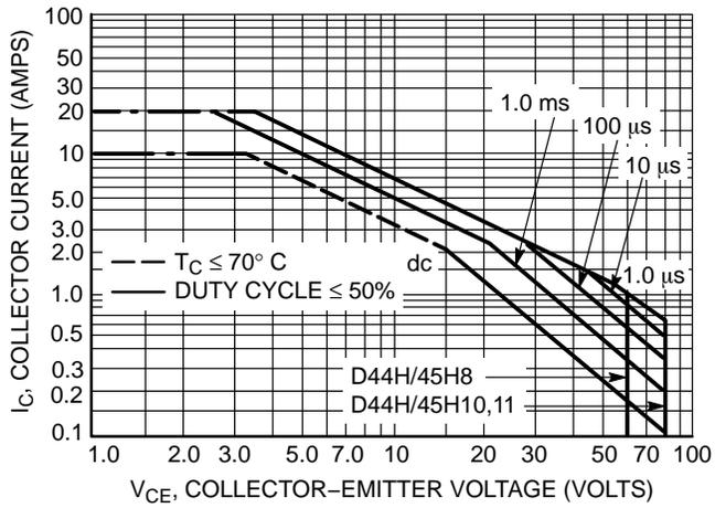
**Figure 9. Maximum Rated Forward Bias Safe Operating Area**
