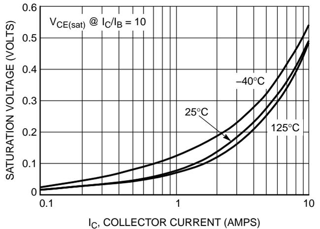
**Figure 6. D45H11 ON-Voltage**
