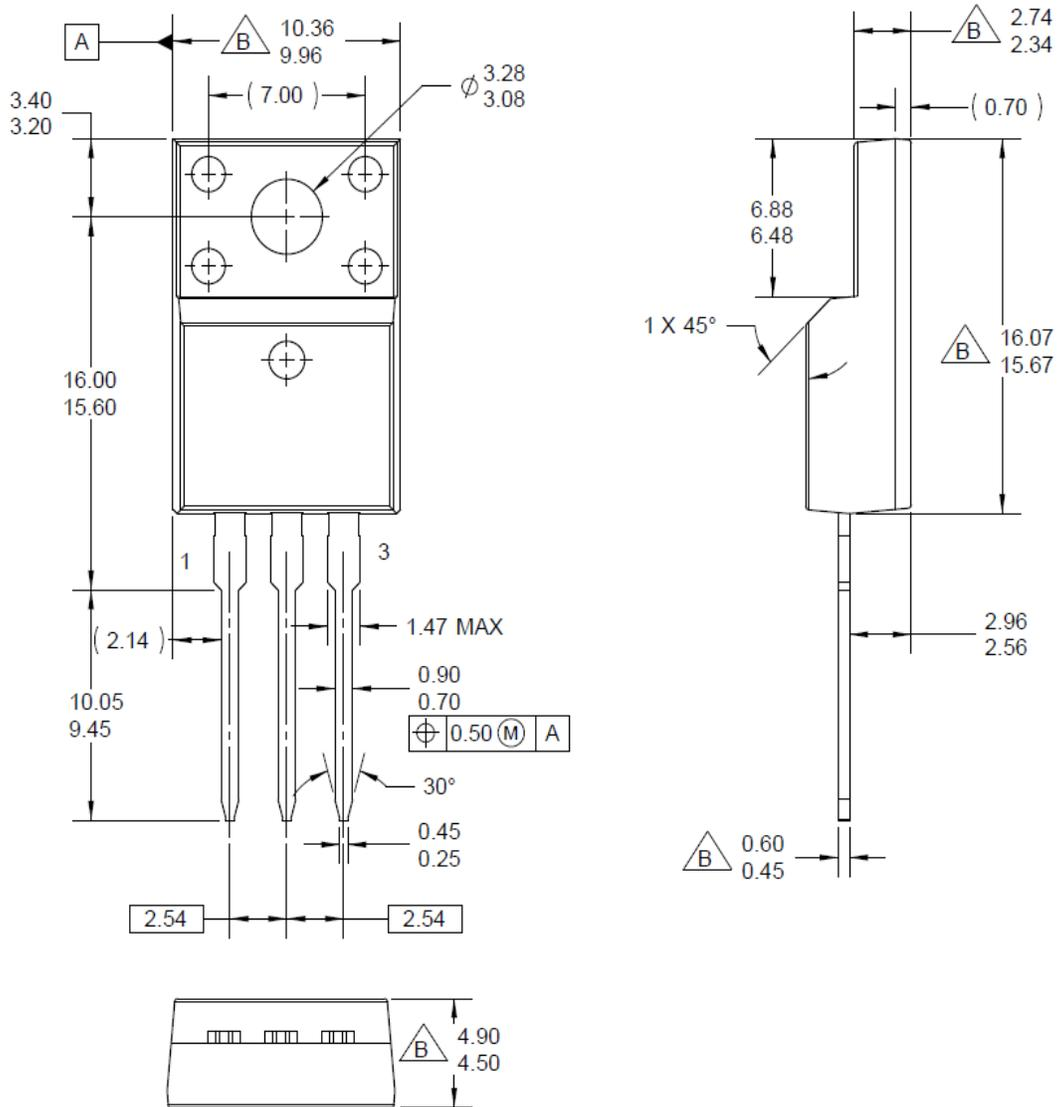
\* Front/Back Side Isolation Voltage : AC 2500V
