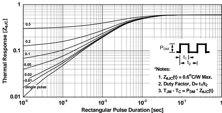
Figure 14. Transient Thermal Response Curve - FCPF190N60
