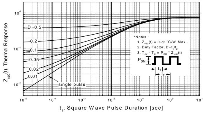
Figure 11-2. Transient Thermal Response Curve (FCPF16N60)
