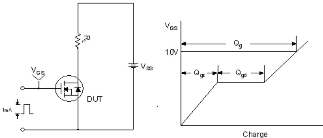
**Resistive Switching Test Circuit & Waveforms**
