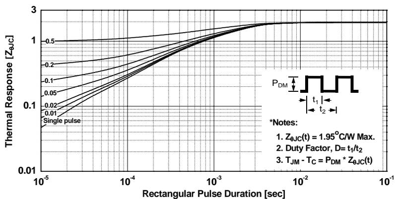
Figure 13. Transient Thermal Response Curve \_ FCPF7N60NT
