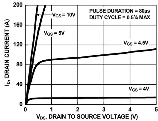
Figure 8. Saturation Characteristics
