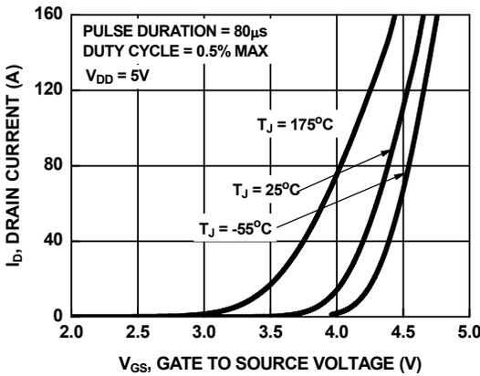
Figure 7. Transfer Characteristics
