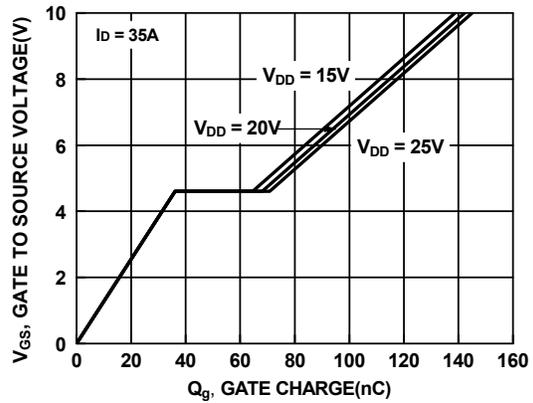
Figure 14. Gate Charge vs Gate to Source Voltage
