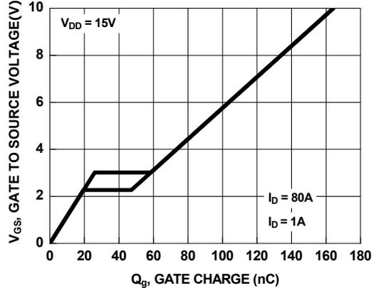
**Figure 14. Gate Charge vs Gate to Source Voltage**
