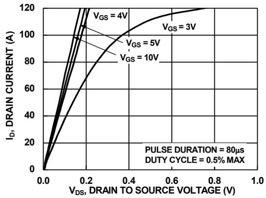
**Figure 8. Saturation Characteristics**
