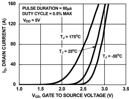
**Figure 7. Transfer Characteristics**
