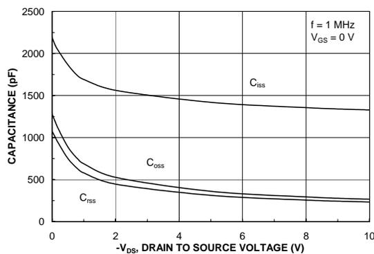
Figure 8. Capacitance Characteristics.
