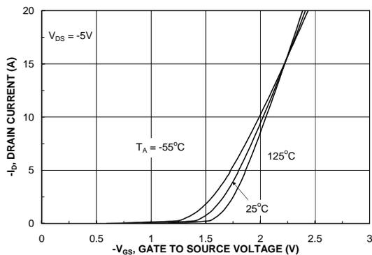
Figure 5. Transfer Characteristics.
