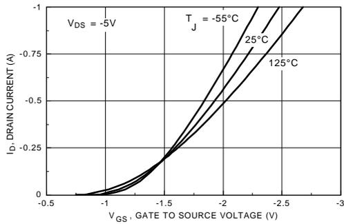
Figure 5. Transfer Characteristics.
