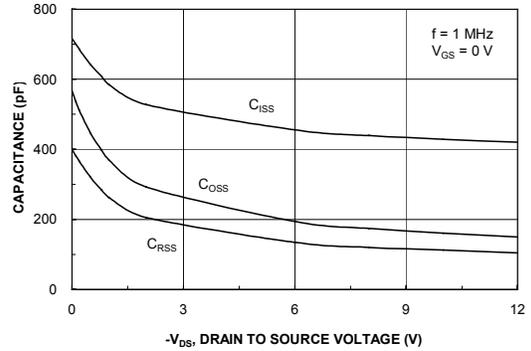
Figure 8. Capacitance Characteristics.
