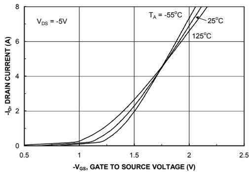
Figure 5. Transfer Characteristics.
