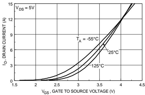
Figure 5. Transfer Characteristics.
