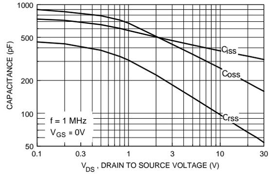
Figure 8. Capacitance Characteristics.
