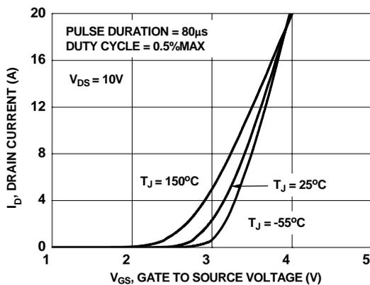
Figure 5. Transfer Characteristics
