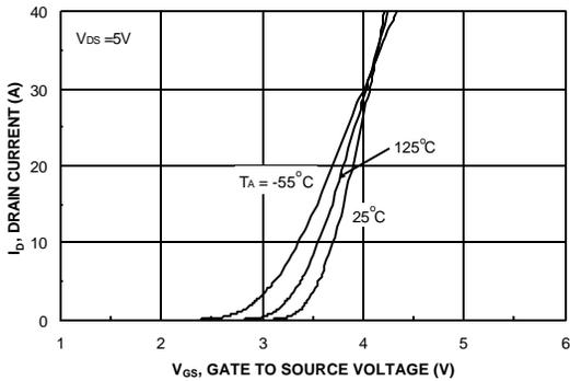
Figure 5. Transfer Characteristics.
