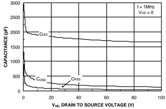
Figure 8. Capacitance Characteristics.
