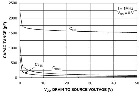
Figure 8. Capacitance Characteristics.
