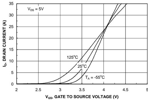
Figure 5. Transfer Characteristics.
